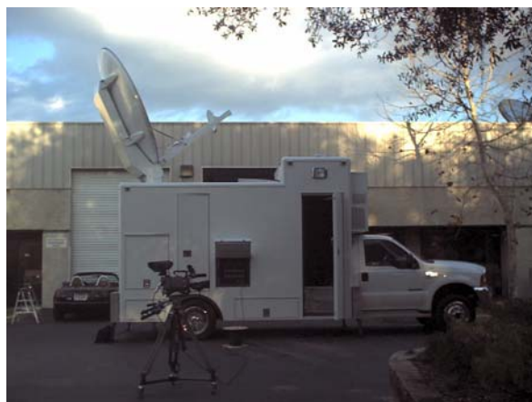
Two-Camera Ku Truck with Mobile Production Ministry of Information, Sultanate of Oman
