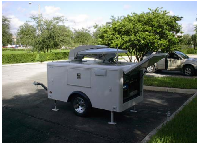
Ku-Band Mini-CMT with Antenna Stowed, Equipment Compartment Open ( wireless version )
