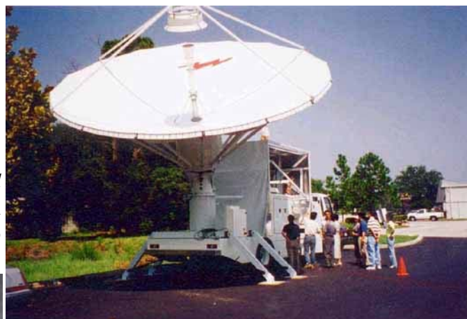
7.3-meter C-Band Truck for Emergency Communications, Beijing, China
