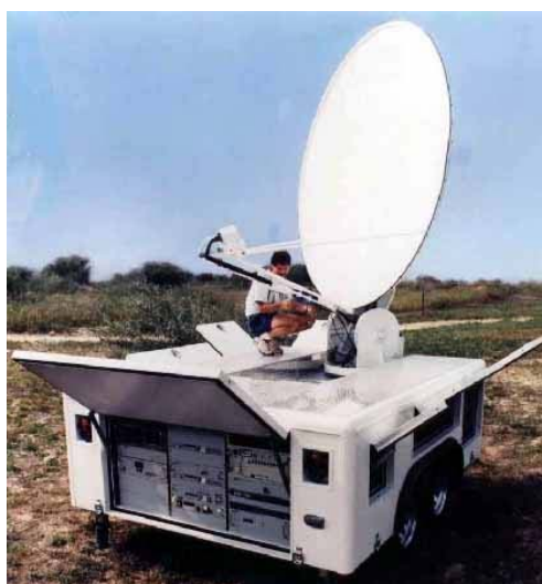
CMT with Antenna Deployed and Equipment Compartment open at rear
